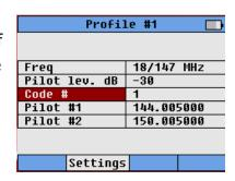
To set this level simply select Pilot level and use the Up and Down arrows to select the desired level relative to the QAM channel.
