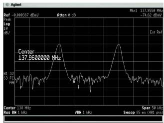
As described above the Pilot/QAM detector utilizes seven codes to set the detector for fixed pilot frequency detection. An eighth code is available for custom setup. To detect carriers like this, use the soft buttons and keypad to select Settings/Leakage detector, then turn the AERO band detection ON and select Pilot/QAM Leak signal.
