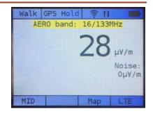
When in Walk mode, the detector will only detect leaks on the one channel that is shown on the display. In the example to the right, the detected leak is measured on the aeronautical band channel 16, centered at 133 MHz. In Walk Mode the detection process is performed two times per second.
