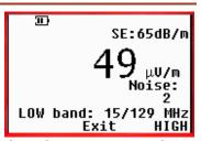
The Nav+ can be configured as a pilot detector to operate at either the aeronautical band and/or the LTE band.
