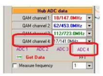
After reading the required precise frequency number, please write it down. This will be the frequency that must be entered into the customized channel settings on the meter.
