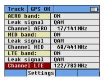
The Mid band is fixed to channels between 201MHz and 645MHz, and the LTE band is fixed to channels between 651MHz and 999MHz.
