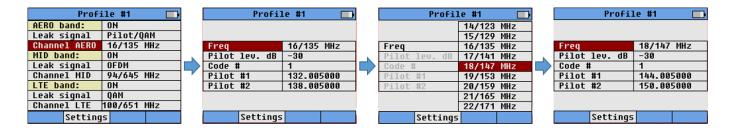
Once Pilot/QAM mode has been selected it is necessary adjust the Detection Code# and level parameters for detection.
