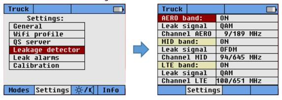
All Navigator Plus devices have at least one local Leakage Detector Profile. Firmware versions N3.15.3 through N3.35.9 have four, which the operator can preset and select as required.
