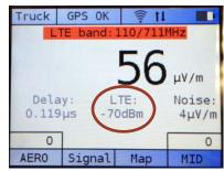
information is then updated to the database each second, and attached to the leak as part of the information used for prioritization. The detected LTE level is displayed in the upper right portion of the screen when the device is cradled. When the device is removed from the cradle, neither the LTE level nor the detected leak level is updated to the database – and LTE level is <u>not</u> displayed on the screen when in walk mode.
