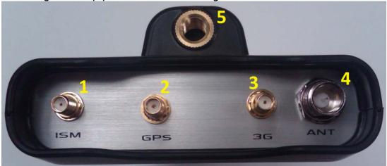
(1) ISM antenna SMA connector input used for transmitting signals to the OAM Snare Isolator
