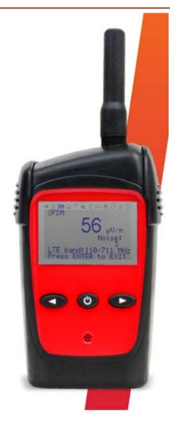
The Snoop Shielding Test detector mode is intended to be used in conjunction with the QAM Snare Pilot Transmitter, to quickly troubleshoot locations in the home and MDU's where poor shielding effectiveness results in forward ingress issues related to close proximity LTE transmitters. Others have referred to this testing technique as 'Pressure Testing'.
