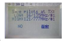
Pilot transmitter setup is a one-time process, and only needs to be repeated if it is desired to change the pilot frequencies.
