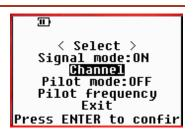
650MHz is considered to be the LTE band. Low band allows selection of OFDM, QAM, Pilot/QAM, Analog, or OFF. LTE band allows selection of OFDM, QAM, or off.
