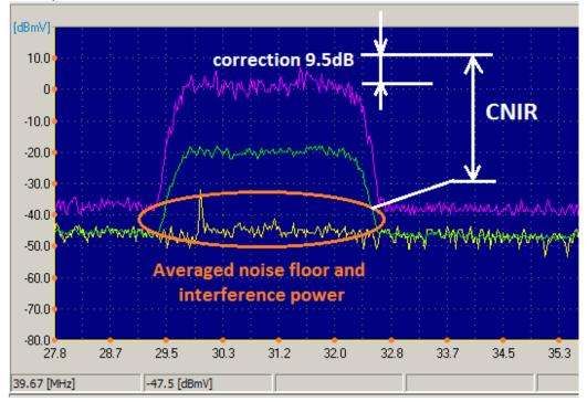
If a peak-like interference is present under the QAM data carrier, the displayed CNR is more accurately described as CNIR (Carrier to Noise + Interference Ratio). Note: power of the QAM carrier and the power of the noise floor + interference power under the QAM channels are used in calculations.
