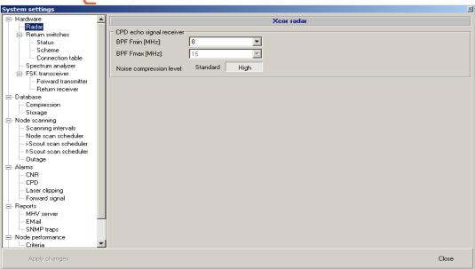
The CPD radar is equipped with a variable bandpass filter. The user can utilize this bandpass filter to select a frequency band which is not affected by strong CW-like carriers that disturb correlation processing of the signals. The lower frequency of the filter band can be switched between 8,9,10.5 and 12MHz.
