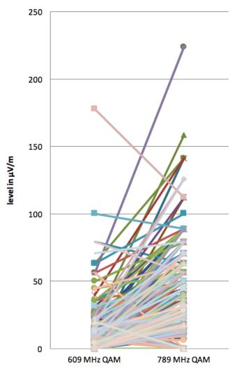
The only trend to take from this data is that in general the majority of lines slope to the left, indicating a higher detected level at the LTE band as compared to 609 MHz. This trend has been observed in various locations. There are simply more leaks, and at greater level, the higher in frequency that you detect.
